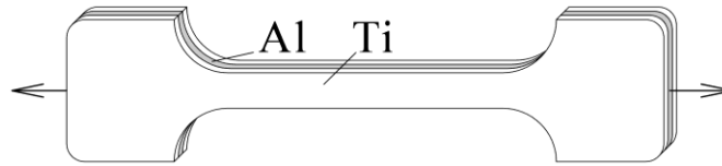
Fig. 3. Schematic representation of a specimen for tensile tests
