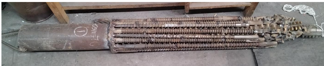
Figure 2 View of the prepared electrodes from the used small tool from steel P6M5
