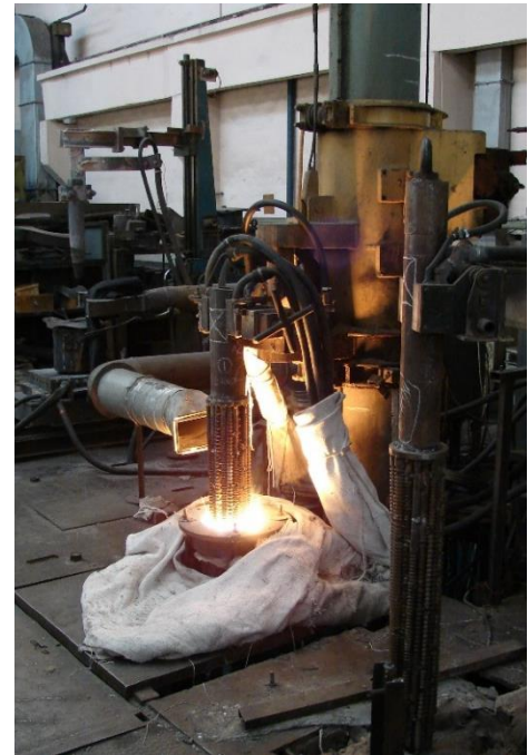
Figure 3 General view of the remelting process of experimental electrodes made of used tool steel P6M5
